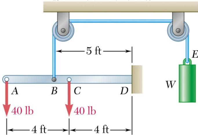
Beam AD carries the two 40 lb loads shown. The beam is held by a fixed support at D and by the cable BE that is attached to the counterweight W. Determine the reaction at D when (a)  $W = 100$  lb, (b)  $W = 90$  lb.
