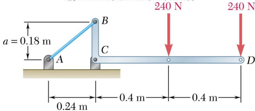
The bracket BCD is hinged at C and attached to a control cable at B. For the loading shown, determine (a) the tension in the cable, (b) the reaction at C.
