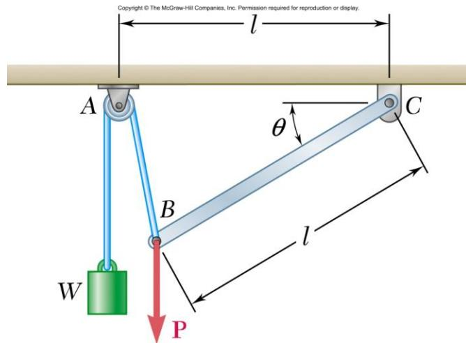
A vertical load  $P$  is applied at end  $B$  of rod  $BC$ . (a) Neglecting the weight of the rod, express the angle  $\theta$  corresponding to the equilibrium position in terms of  $l$ ,  $P$ , and  $W$ . (b) Determine the value of  $\theta$  if  $P = 2W$ .
